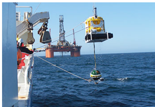
seismometer (below the yellow flotation unit) measures underground vibrations on the sea bed. Spectraseis uses its technology to evaluate the vast quantity of seismic data generated. Photo: Spectraseis
