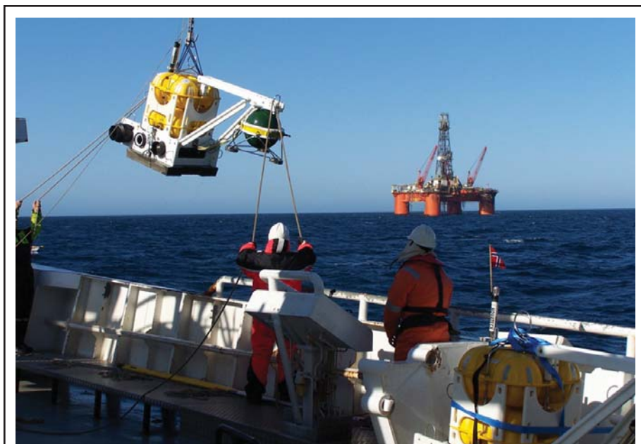
Recoverable ocean-bottom sensors can be deployed offshore to acquire marine passive seismic data. A pilot program conducted in the Gulf of Mexico demonstrated that low-frequency anomalies in the seismic data are related to the presence of hydrocarbons.
