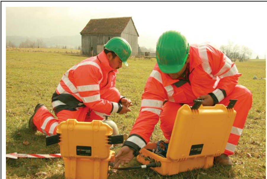
Low-frequency passive seismic technology is helping to improve the value of conventional seismic data by overlaying structural interpretations with reservoir information, and is giving surveying crews the ability to acquire data off limits to traditional exploration. Shown here, a seismic crew deploys equipment to conduct a passive low-frequency spectral analysis survey in Austria.
